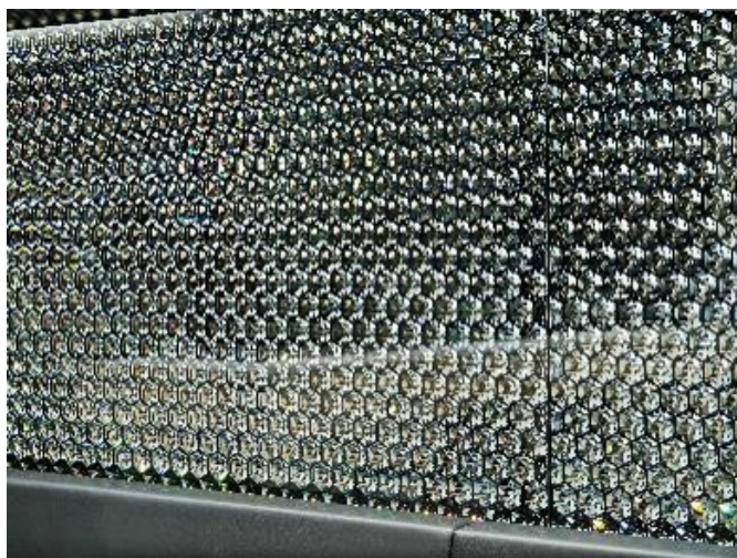
Figure 20: A hexagon panel using freeform microstructured foils/plates with a gemstone appearance.
